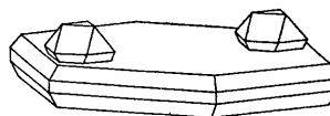
Fig. 1. Habit of hexagonal barium titanate and coalescence of octahedral faces of small cubic crystals on hexagonal basal face.
