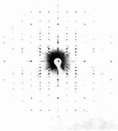
Fig. 4. The h0,l layer of the reciprocal lattice. Reciprocal a axis horizontal, reciprocal c axis vertical.
